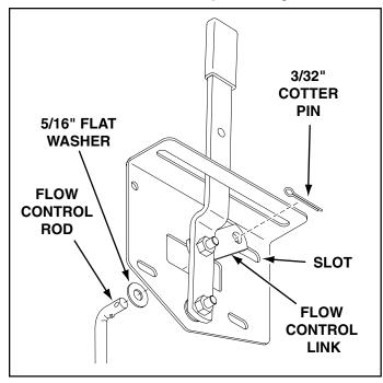
19. Hook the free end of the flow control rod through the hole in the slide gate bracket located near the bottom of the hopper. See figure 10.
